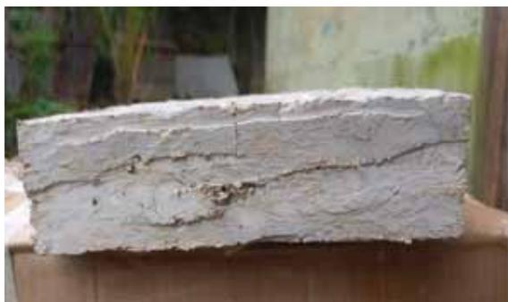
**T3 (Cemento 60% + Fibra 40%)**
